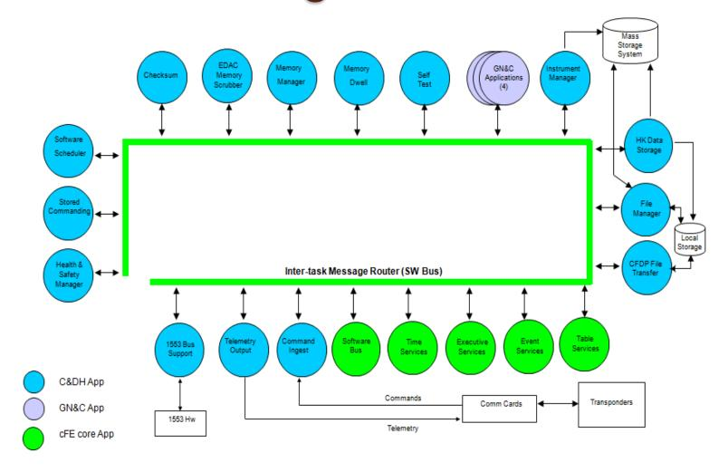
"Lollipop" Diagram shows cFE core applications and software bus (green), plus CFS applications that plug into the bus (blue and purple).
