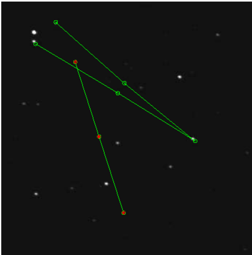
Left: Trajectory Detection for the CSS Triplet. Right: Trajectory Detection for the CSS quadruplet. Asteroid trajectory detected is shown in green. True location is in red.
