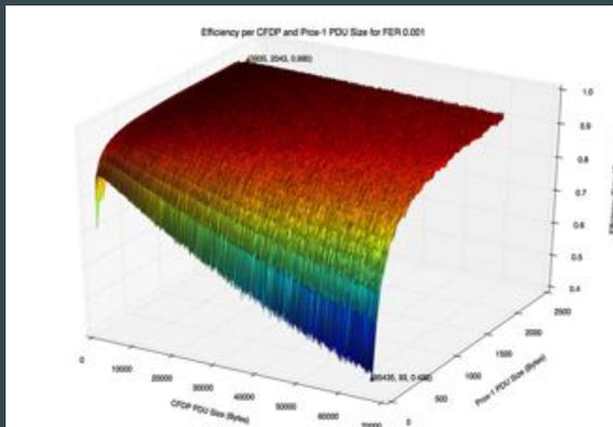
On lossy links, efficiency quickly degrades with increasing PDU size.
